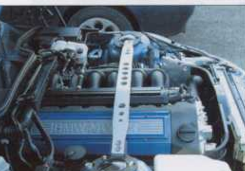
The authors gleaming engine bay, complete with colour coded cam cover and 'strong strut' brace
